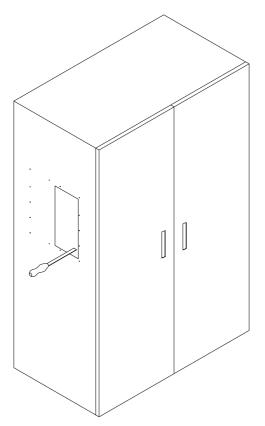
10. Put the socket plug in the position and screw it <u>be careful</u> the socket plug cover must be opened up only
