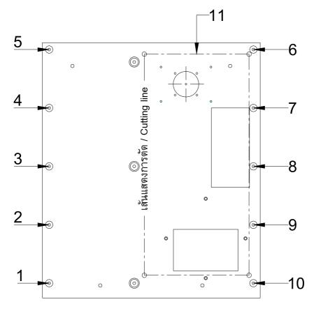
3. Cover eqipments inside cabinet with clean and dry cloth,and cover with paper boxes at position will be drilled and cutted in order to prevent metal scrapt falling in cabinet.
