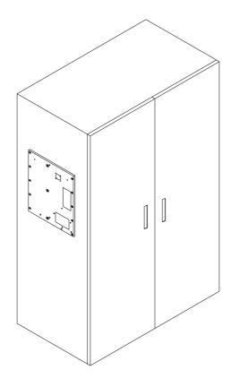
2 Layou 10 posittion for drilling and cutout along the dot line with Jigsaw
